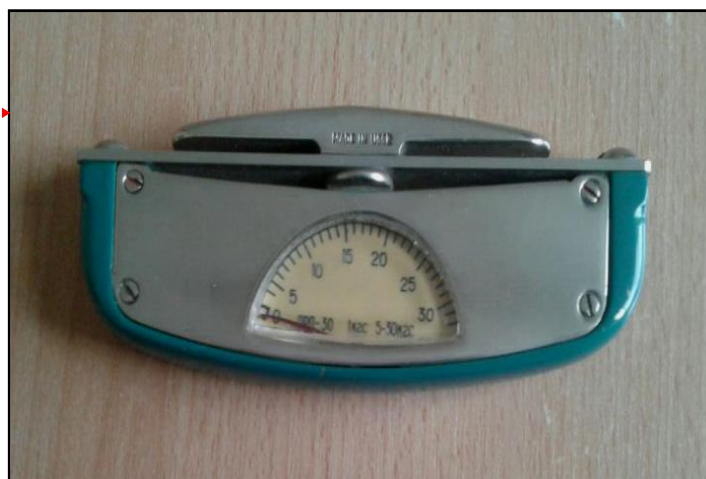
Figure 2.Measuring hand strength (kg) in elementary school students using a dynamometer (DPR-30).
