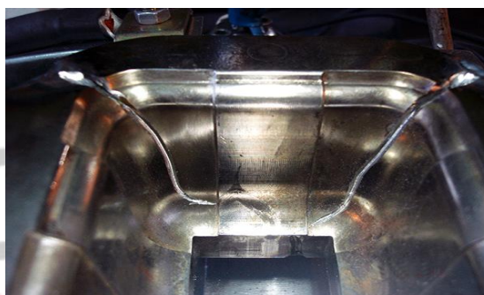
Figure 6. Detection of cracks in the corners of the press-mould matrix
