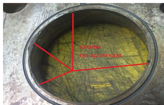
Figure 4. This matrix is a view of the worn edges of the punched plates of the Puanson press mould.
