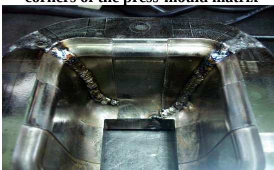
Figure 8. The technology of filling of forming surfaces by filling methods
