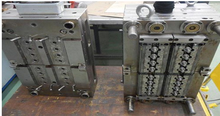
Figure 9. External inspection of forming joints and press-mold parts
