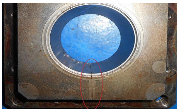
Figure 3. Cracks in matrices.
