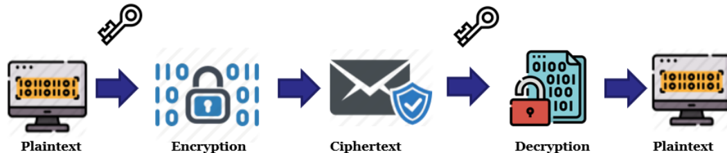
FIGURE 2. Symmetric key cryptographic system
