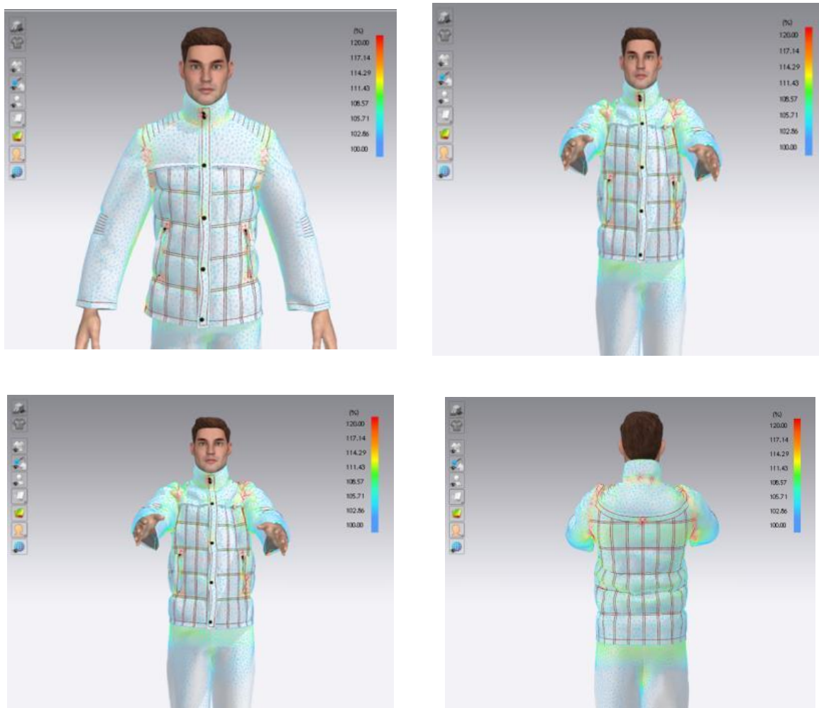
Figure 4. The parts of the men's jacket that are most susceptible to mechanical stress in the CLO D3 program
