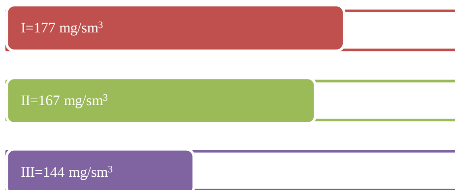
Figure 2. Variation in bulk density of knitted fabric with pattern
