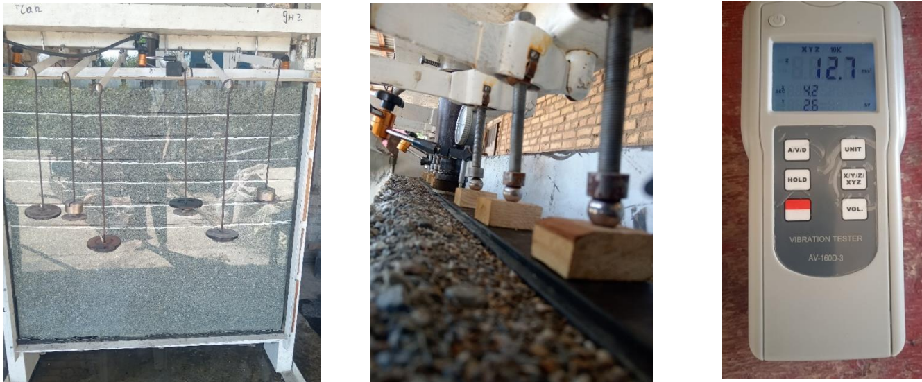
FIGURE 2. Dynamic analysis results for a 1-meter long beam with a base of Sheben soil
