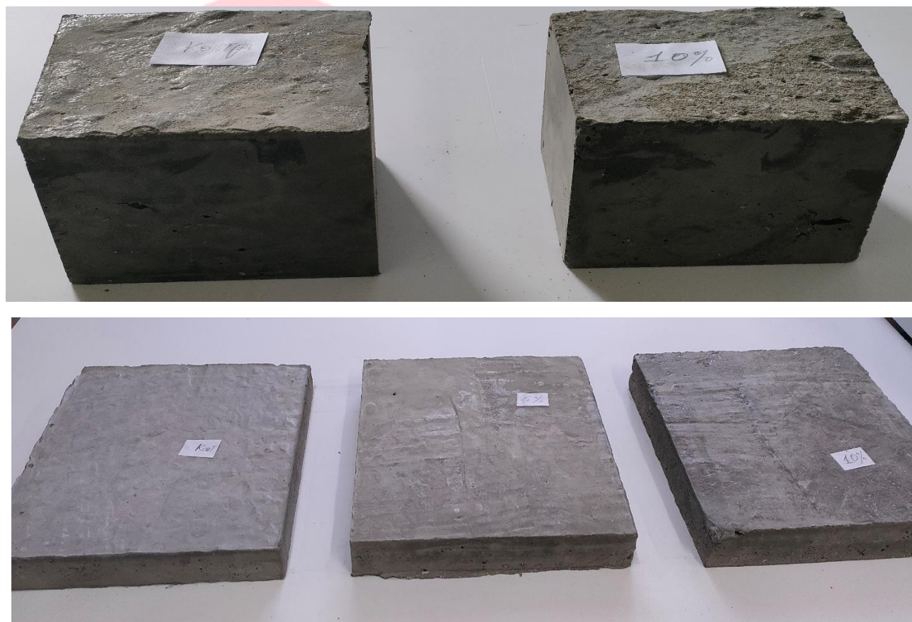
Figure 1. Samples of concrete prepared on the basis of wollastonite and vermiculite minerals.
