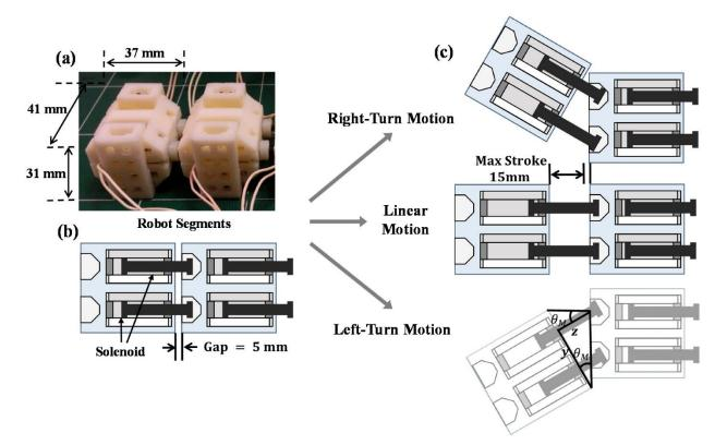
Prototype Fabrication: Based on the results of the conceptual design exploration, a prototype of the MagPlunge solenoid actuator was fabricated. This involved the selection of appropriate materials,
