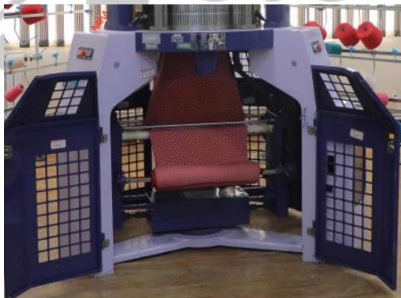
Figure 5. Pulling and wrapping system
